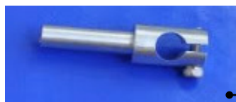
REDESIGNED SHAFT OILER Designed for the 11/32 inch brass tube
